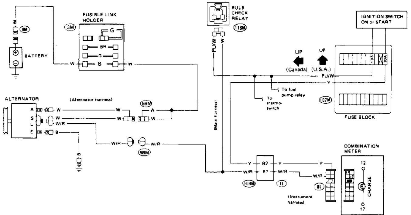
Fig. 3: Pulsar NX Charging System Wiring Schematic (Others Similar)
