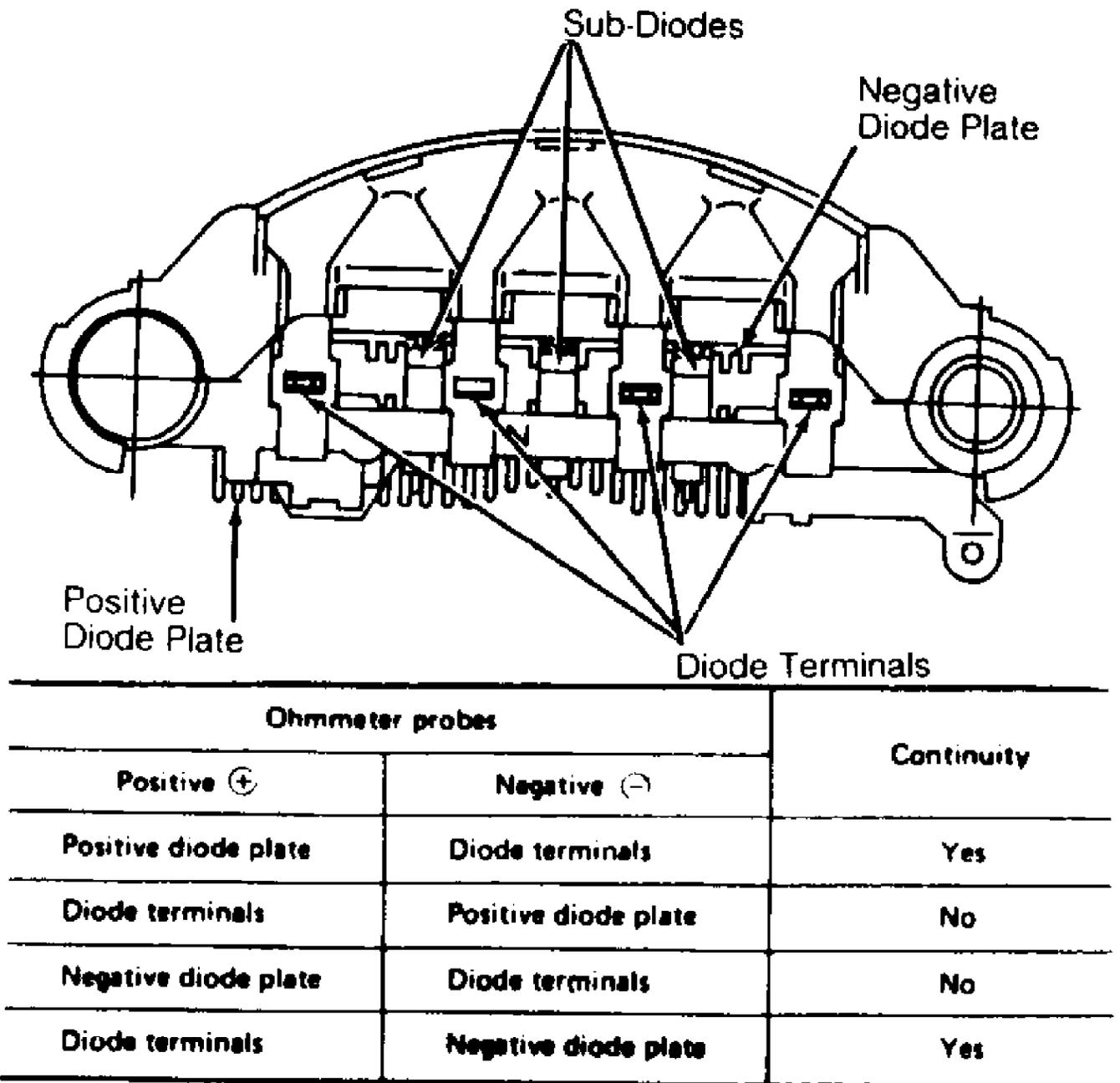
Fig. 1: Testing Diode Assembly
