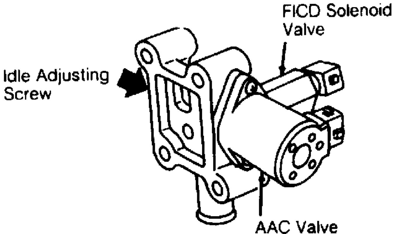
Fig. 3: Adjusting Idle Speed (240SX)
