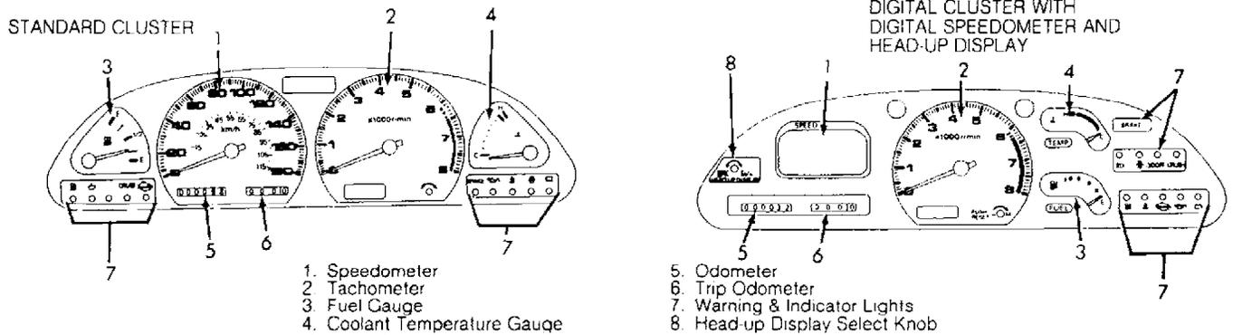
Fig. 1: Dash Gauges & Warning Lights
