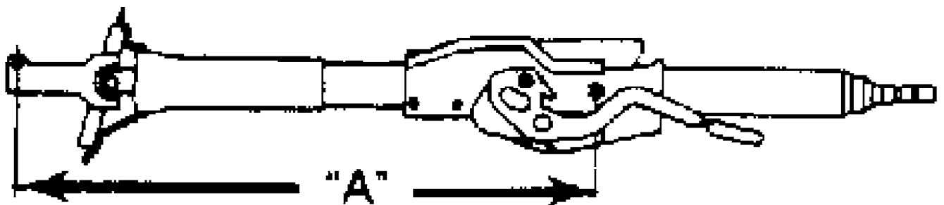
Fig. 5: Steering Column Measuring Points (Stanza) Courtesy of Nissan Motor Co., U.S.A.
